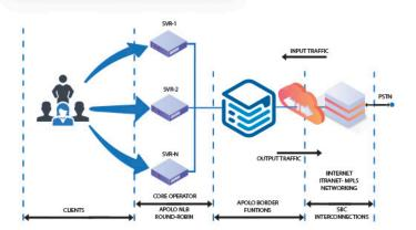
Apolo Switch SBC can be applied in different scenarios preserving the security functionalities, integrity of the SIP Protocol and handling of RTP Packets.
